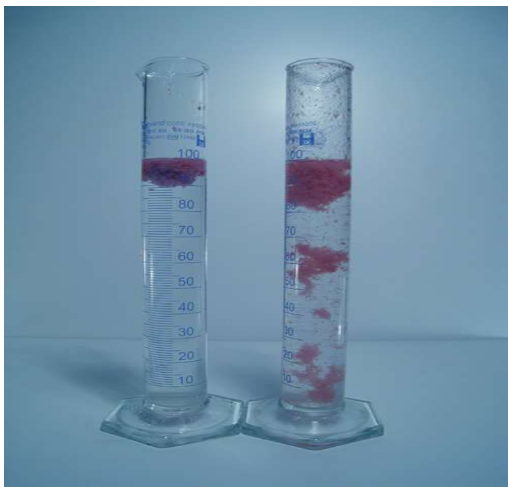
Figure 19 : Traitement coagulation- flocculation
